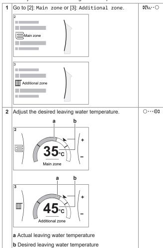
To change the weather-dependent curve for the space heating/cooling zones
